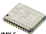
IMX-6 Size: 15.6 x 12.5 x 2.9 mm Weight: 0.9 g INS: External GNSS Input
